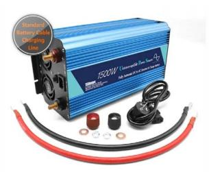
BET1500S is a household, office multi-functional UPS inverter, through the distribution of battery lines and battery links can provide maximum 1500W rated power and 3000W peak power. BET1500S can be connected to the mains to charge the batteries and provide automatic switching between the mains and the batteries. At the same time, it can provide stable AC voltage input. The power cord is made of multi-core oxygen-free copper, and the power supply with large load is guaranteed.
